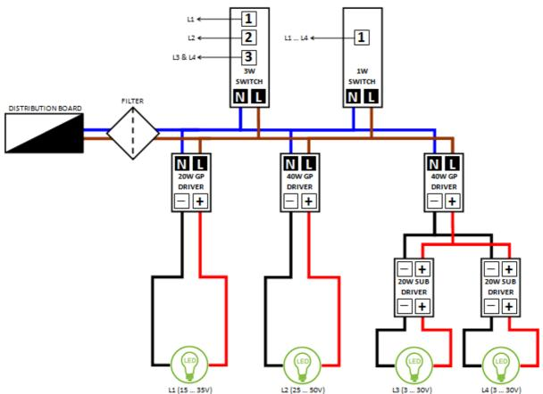
The switches are supplied with 2 connections ; Phase (red) and Neutral (black) and are wired to a quick connect block. Wiring into this block can be 1.0mm, 1.5mm or 2.5mm TPS cable. An earth is not required.
